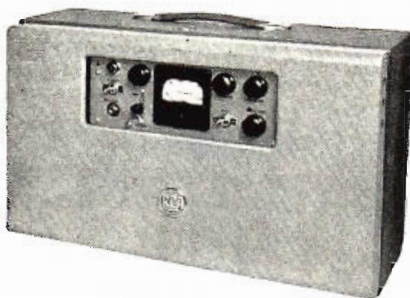
THE RELAY RECEIVER consists of the receiver unit itself, which is mounted on the rear of a parabolic reflector (and is similar in appearance to the transmitter unit) plus the receiver control unit shown above. The parabolic and receiver can be mounted on a permanent structure as shown at the top of this page or on a tripod similar to that used with the transmitter. The control unit is assembled on a bathtub-type chassis (top) which can be mounted on a standard rack or in a portable carrying case (bottom).
